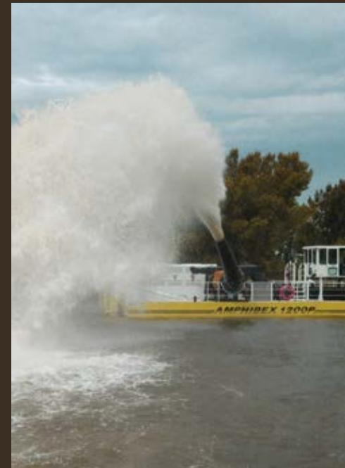
The Amphibex 1200P will meet your high expectations in volume: dredging (contaminated sediment, mud or sand); pipeline installation; underwater cables; pile driving; controlling aquatic plants. The dredging capacity is between 42,000 to 44,000 GPM.
