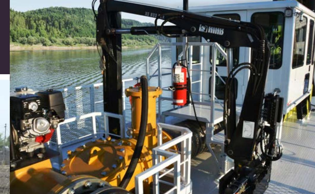
The Amphibex 850P will meet your high expectations in volume: dredging (contaminated sediment, mud or sand); pipeline installation; underwater cables; pile driving; controlling aquatic plants. The dredging capacity is between 18,000 to 20,000 GPM.
