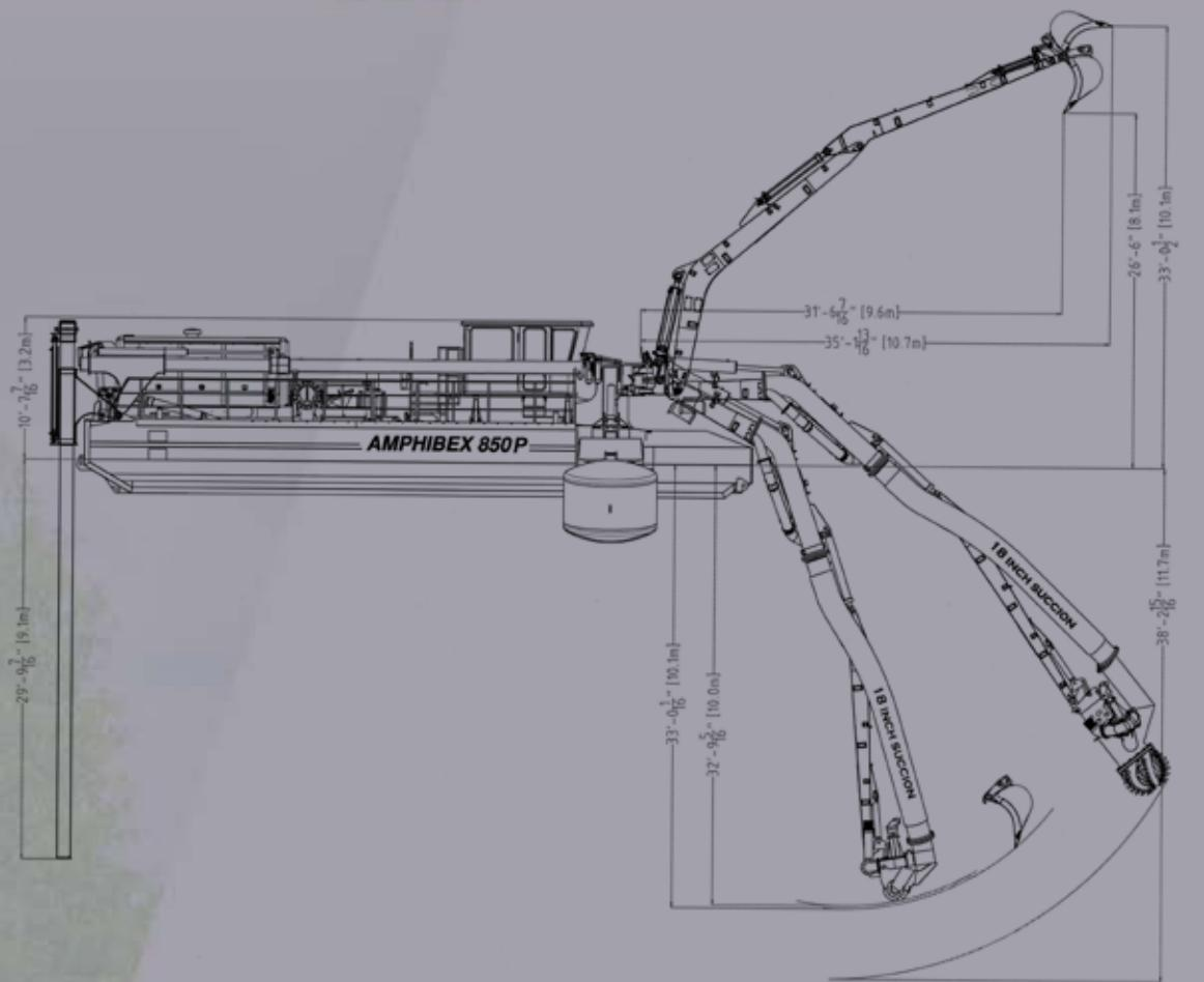
The maximum length of the Amphibex 850P is 15.4 meters and its maximum width is 4.3 meters. It can move at a speed of 5 to 8 knots. Its diesel motor is a model C18 6 cylinder Caterpillar, with 765 hp, and a diesel tank of 3140 litres.
