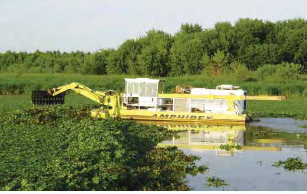
Cleaning and restoring waterways; cleaning ponds; controlling vegetation; creating wildlife habitats; installing water pipes, pipelines and underwater cables; preventing and breaking ice jams; developing peat lands. These are just a few of the things you can do with the Amphibex 400.
