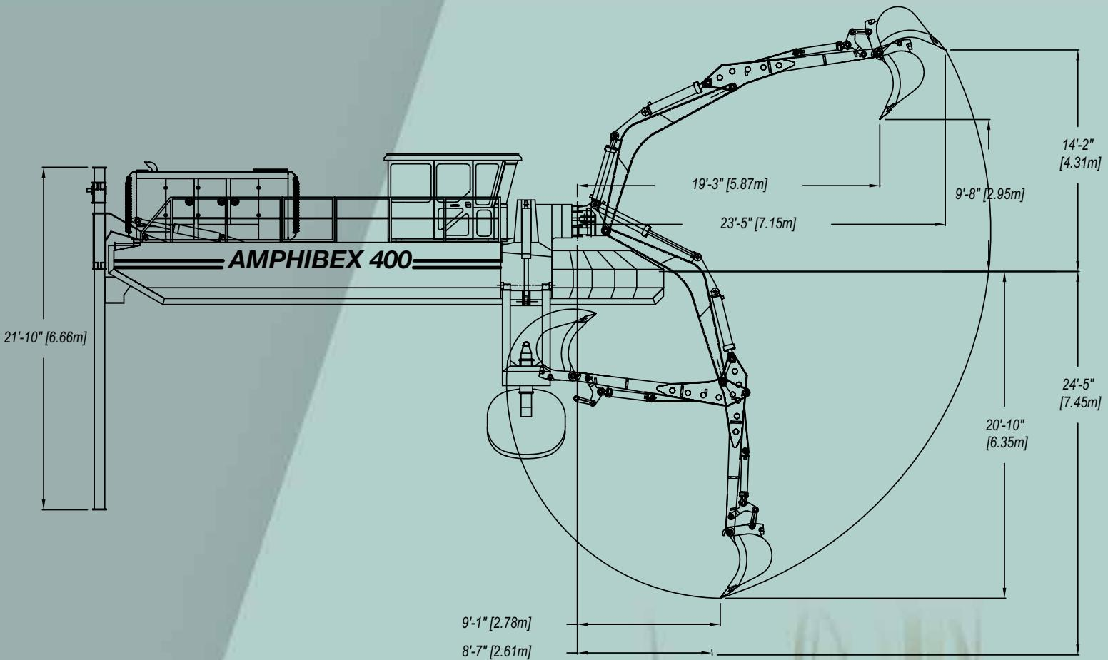
The maximal length of the Amphibex 400 is 10,85 meters and total weight is 22 tons. It can reach a sailing speed of 5 to 8 knots. The diesel engine is a six cylinder Caterpillar C9 with 350 hp. The hydraulic system has a capacity of 500 litres, runs on vegetable oil and feeds five pumps (one compensated pressure and four variable flow).
