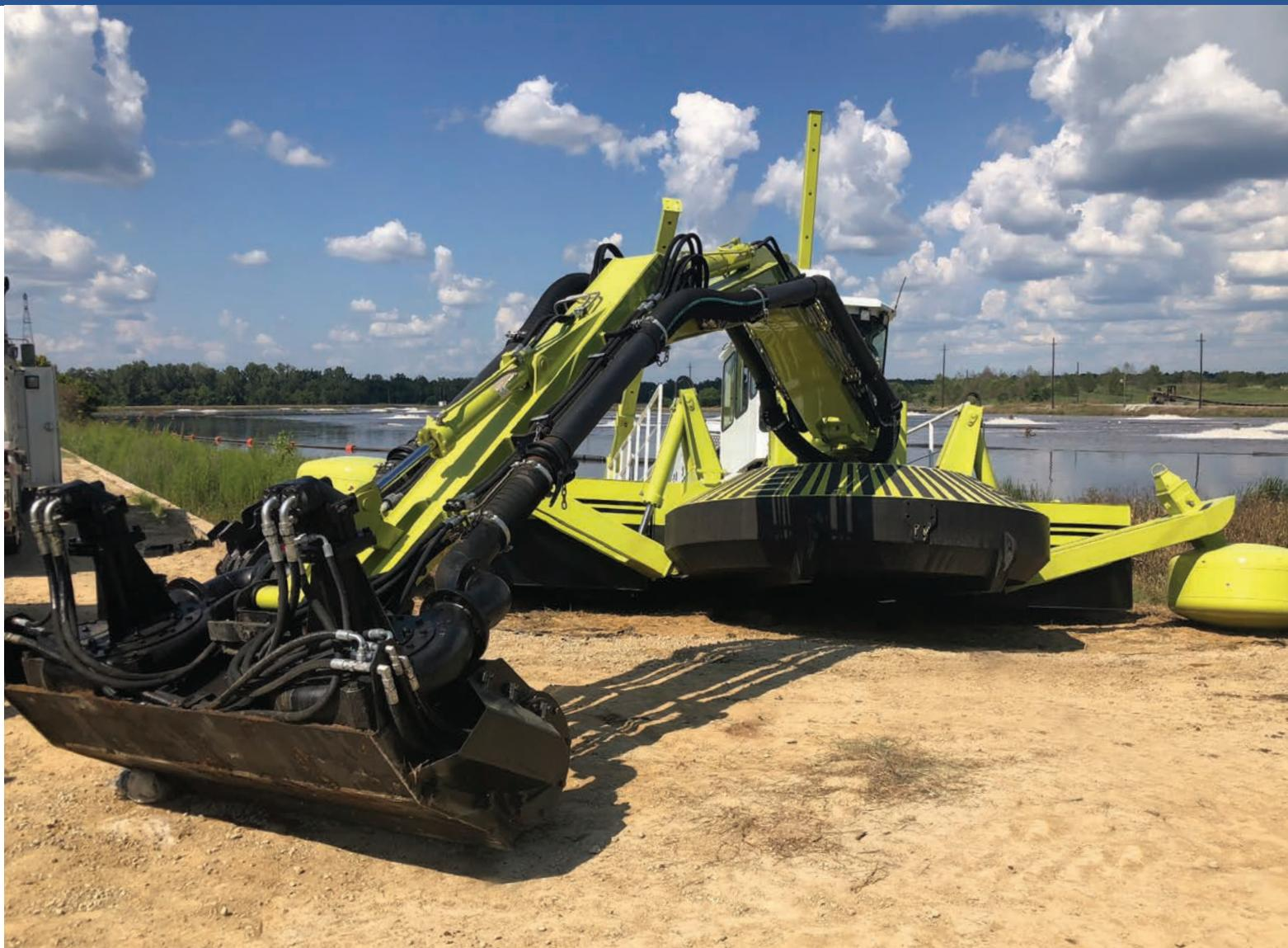
The Amphibex 450: specifically designed to operate in aquatic environments. Strong, sophisticated, versatile and safe for the environment. The front stabilizers, equipped with detachable floats and rear stabilizers, equipped with hydraulic tilting cylinders, give this machine its balance, stability and mobility. Amphibex 450 lets you work without damaging the ecosystem.
