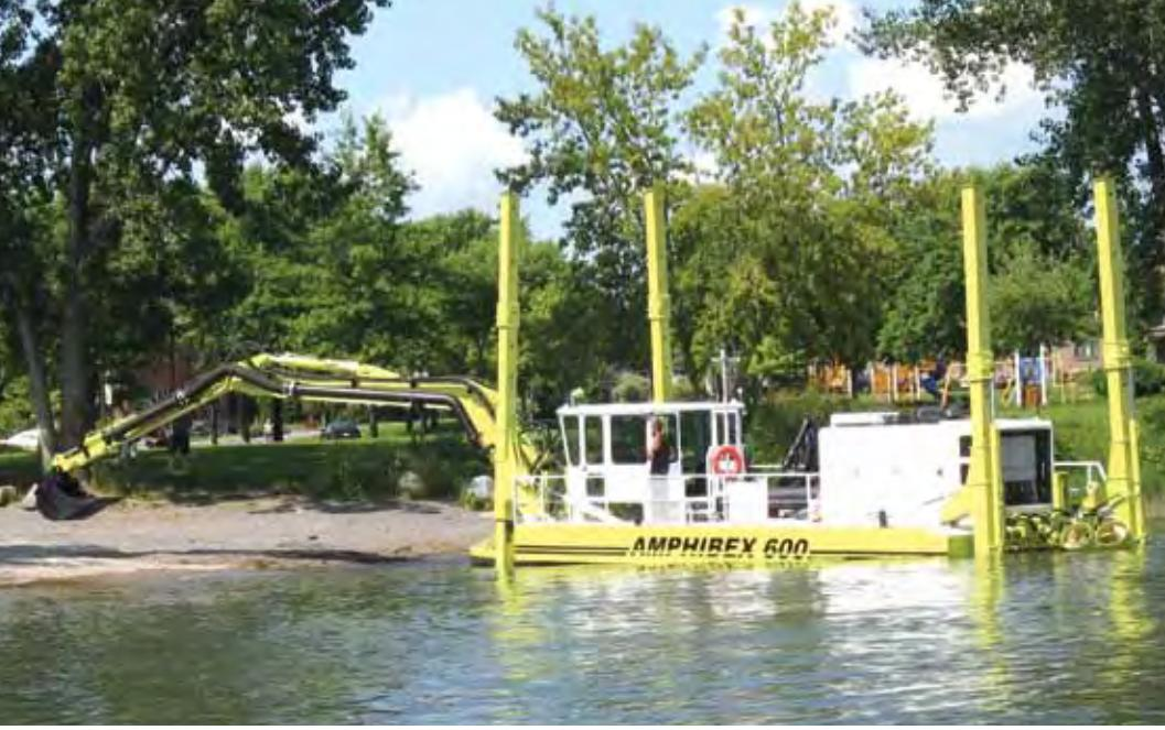
The Amphibex 600 can handle the toughest jobs: dredging (sediment, contaminated sediment, mud or sand); pipeline installation; installation and depression of underwater cables; controlling water vegetation.
