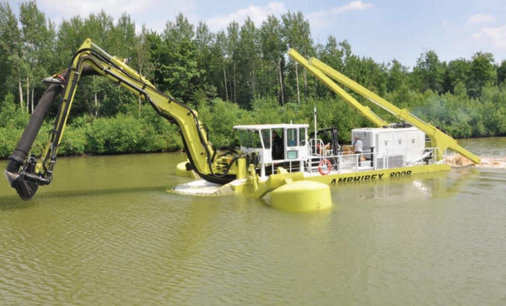
The Amphibex 800P will meet your high expectations in volume: dredging (contaminated sediment, mud or sand); pipeline installation; underwater cables; pile driving; controlling aquatic plants. The dredging capacity is between 18,000 to 20,000 GPM.
