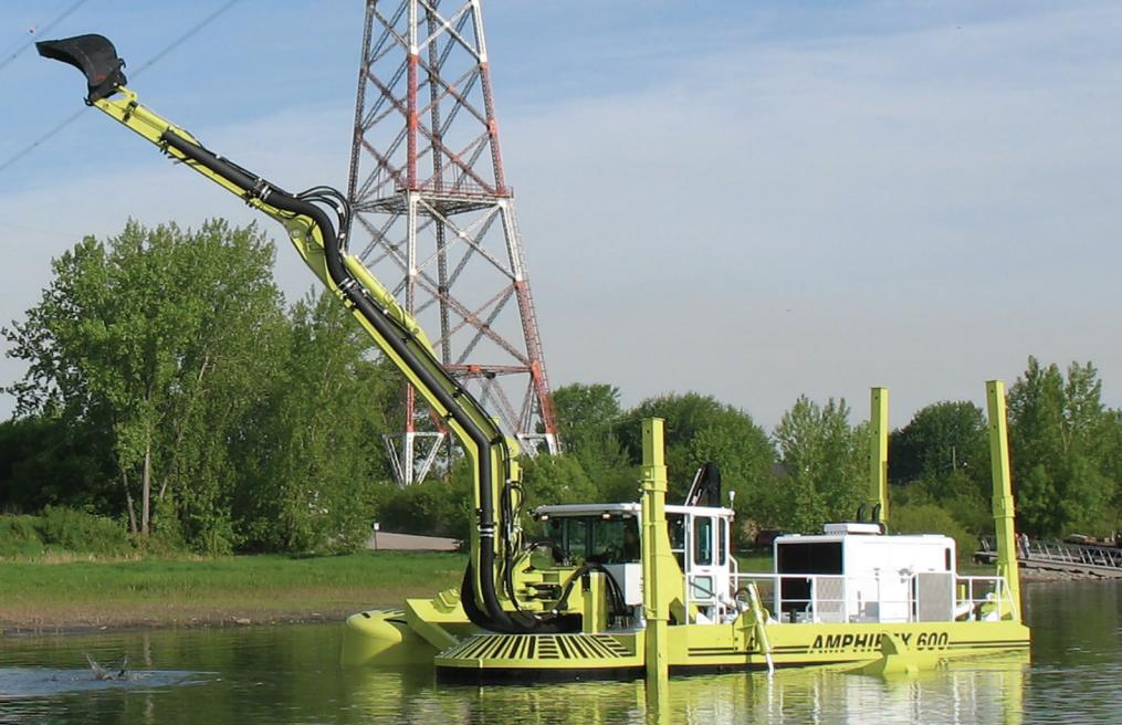
The Amphibex AE650E can handle the toughest jobs: dredging (sediment, contaminated sediment, mud or sand); pipeline installation; installation and depression of underwater cables; controlling water vegetation.
