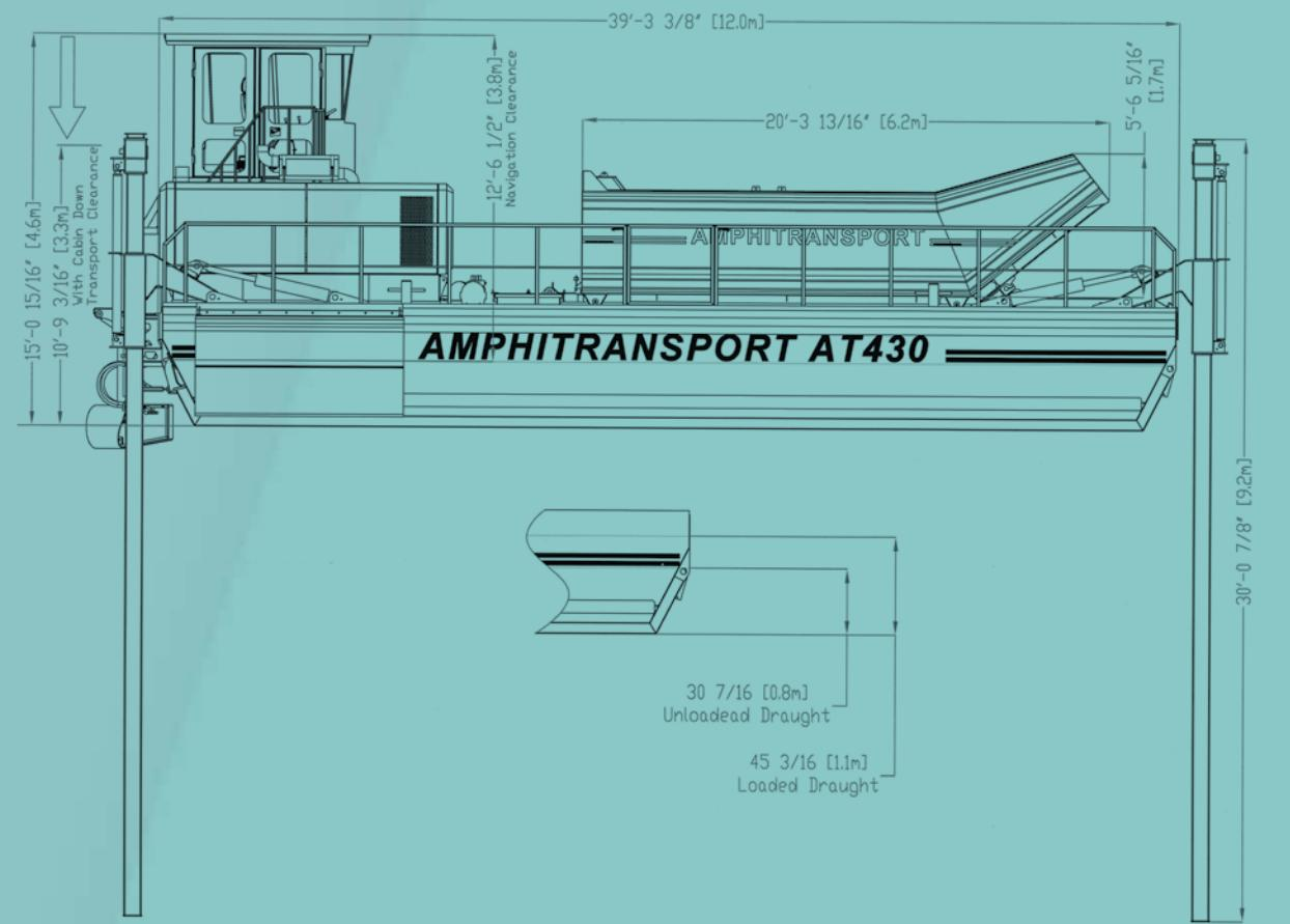
The maximum length of the Amphittransport AT 430 is 12 meters. The engine can move at a speed of 5 to 8 knots in navigation. The engine, a six-cylinder Caterpillar C9 diesel model, generates 350 hp. The hydraulic components include a compensated pressure pump (maximum pressure is 300 bars) and variable displacement pumps (maximum pressure is 420 bars). The system has a capacity of 322 liters.
