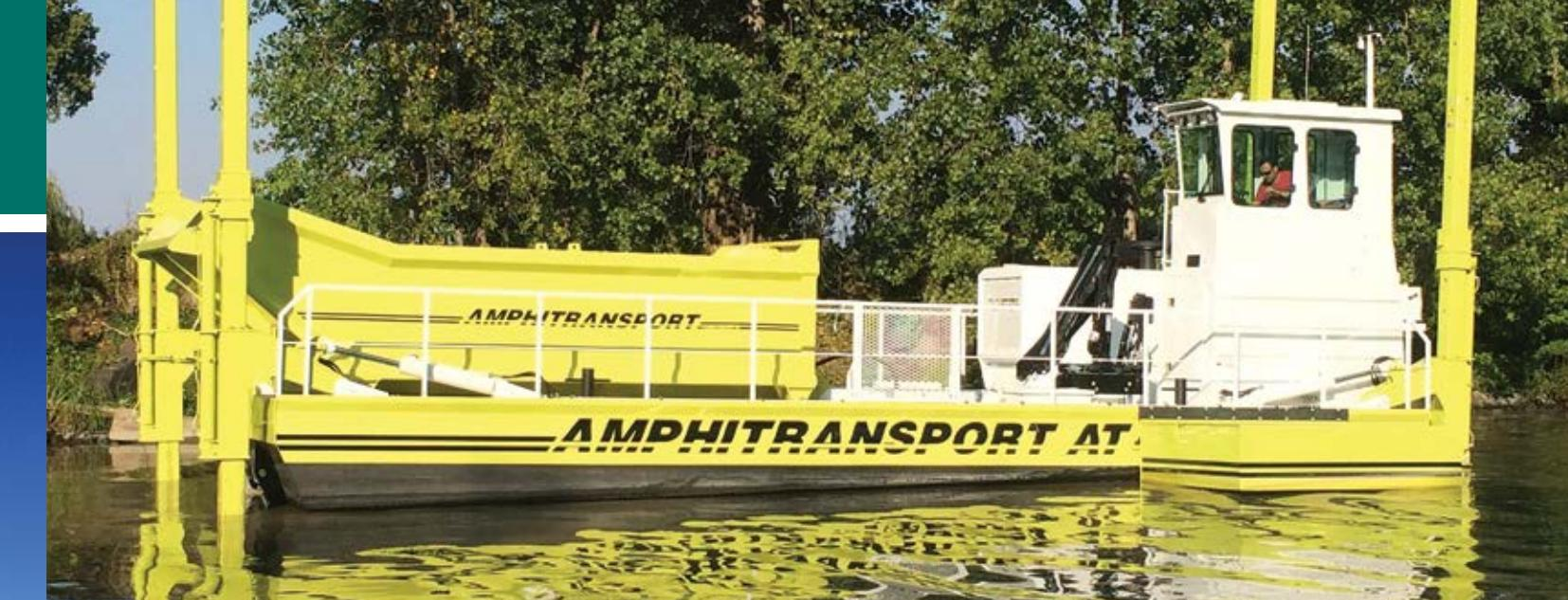
The Amphittransport is equipped with four articulated hydraulic anchor piles which make it possible to work with total stability. The AT 430 moves at a speed of 5 to 8 knots with powerful hydraulic engine propellers. It also moves from the bank to the water without external assistance thanks to these articulated anchor piles.
